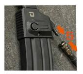
**5.** Pinch and pull the QD ring backwards on the HPA Hose Connector, then attach your "hardware" (could be a AEG magazine adaptor / "HPA Tapped" magazine / Drum magazine / HPA Engine etc to the connector then release the QD ring to its original position.
