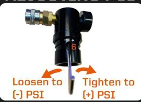
**6.** Loosen the PRESSURE ADJUST-MENT screw with Hex Key anti-clockwise to decrease (-) PSI / Tighten screw clockwise to increase (+) PSI
